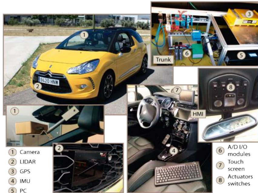
Figure 10 – CSIC's automated vehicle: Sensors and equipment.
